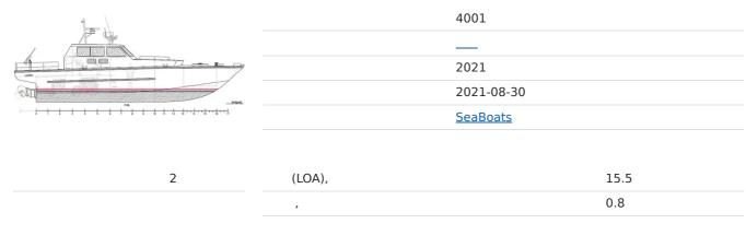
2x Scania DI16 077M 846kW @ 2300 rpm. Propulsion: 2x Doen DJ170HP
